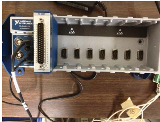
Figure B.1: Proper Location for the NI 9237 Module in the NI chaise
