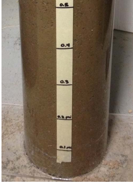
Figure B.20: Shows the bottom half of the calibration test cylinder. Also shows the incremental pressure markings along the outside of the calibration test cylinder.
